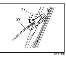
2) Squeeze lock lever (1) towards wiper arm (2) and remove the wiper frame from the arm as shown.
